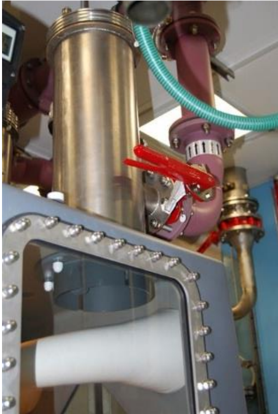
Photo 8. Style A Housing (The device to prevent the filter moving down the housing can be seen through the window). Note: This is a coated glovebox with the filter housing internally coated)
