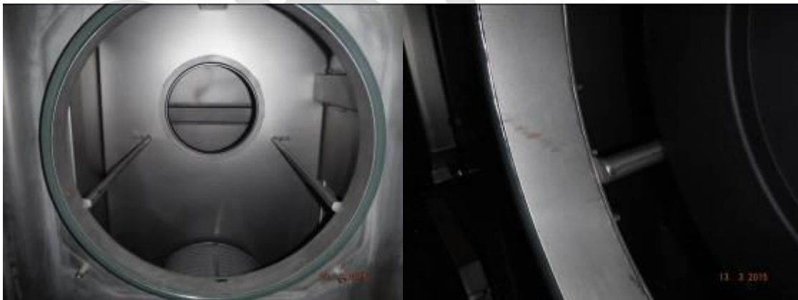
Photos 5 and 6. Guide Rails With Insufficient Corner Rounding
